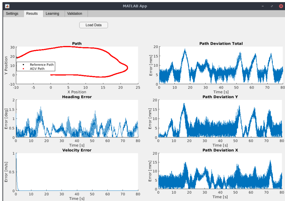
Figure 39: Performance of the PPO agent during one simulation.
