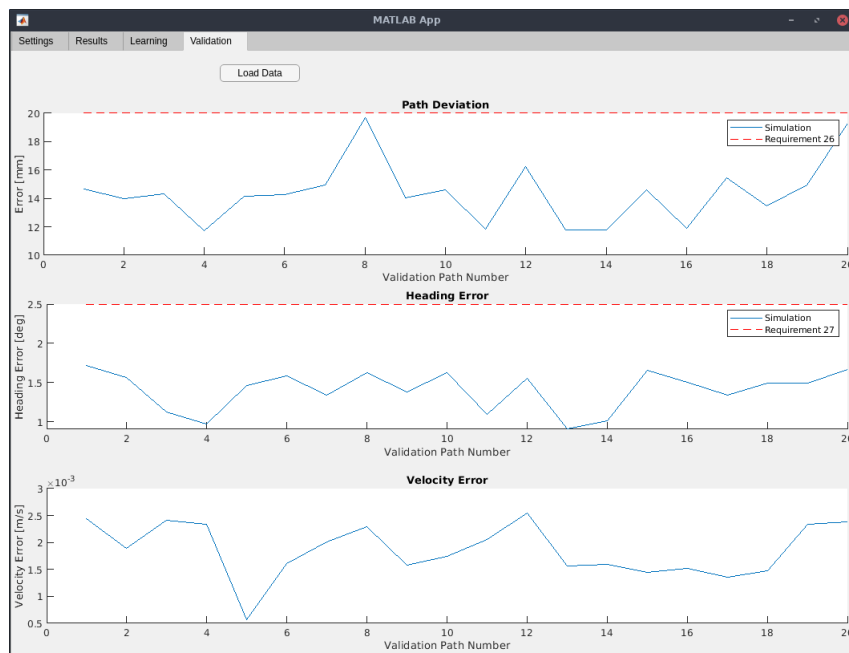
Figure 37: Validation results for the PPO agent for v = 1 m/s.
