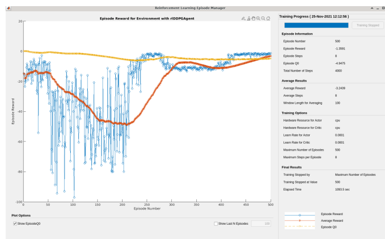
Figure 11: Illustration of the training of the DDPG auto-tuner. The Figure shows the different rewards for the episodes during the training process which indicates different control parameters in the different episodes.
