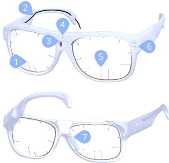
Figure 2: Tobii Pro 3 glasses components. Image rights: Tobii Pro AB
