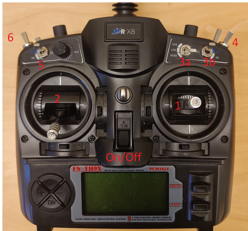
Figure 2: The RC-controller used to fly the UAV, with markings for all the used switches.
