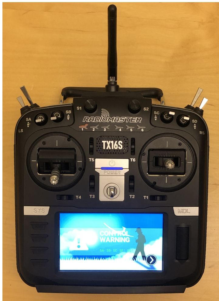
Figure 2: The remote controller from above. The left and right joystick are used to maneuver the UAS
