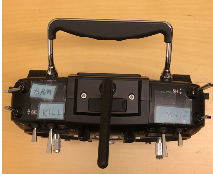
Figure 3: The remote controllers switches. The switches are labeled ARM , KILL and Mode
