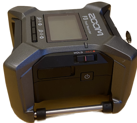
Figure 5: Image of the sound card, showing the location of the record switch.
