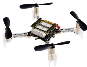
Figure 2: A crazyflie drone, version 2.0.
