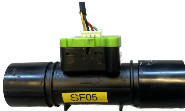
Figure 5: The air flow sensor used in the experiments.
