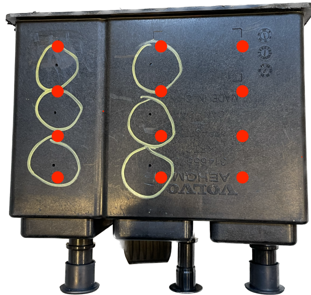
Figure 6: Picture of the canister with temperature sensor placements illustrated by the red dots.
