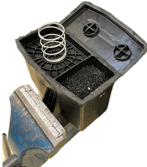
Figure 3: Canister containing activated carbon separated from the bottom. The spring and plate compressing the active carbon can be seen to the left and the activated carbon in the right chamber.
