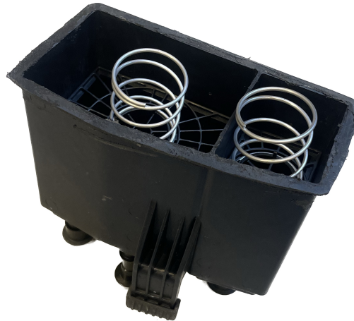
Figure 2: Canister seen from below with springs that keep the active carbon packed inside the canister. The bottom piece of the canister is missing in this picture.
